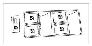
The power window switches are located on the armrest near each window. Press the front of the switch to the first position to open the window to the desired level. Lift up the front of the switch to the first position to close the window.
